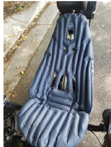
Above: Front suspension showcases more examples of beautiful machine work and design and provides a delightful ride. Left: Seating on the Triot is a unique inflatable bladder design over a padded carbon-fiber shell.
