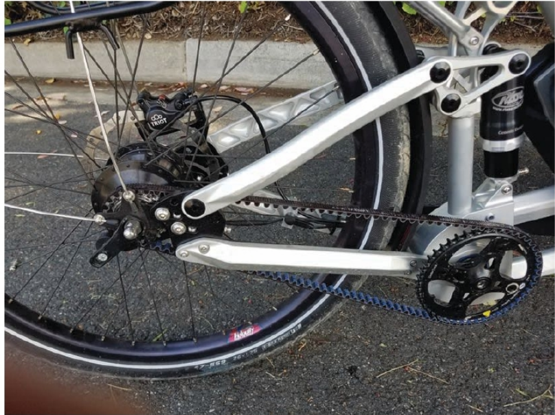
Above: Final drive is provided via a silent-running belt drive, the five seat back positions can be seen above the suspension shock. Rear hub is a 14-speed Rohloff with electronic shifting. Below: Easy to read computer screen shows all the relevant settings selected via touch buttons on the handlebars.
