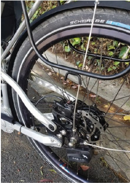
Mr. Zupke found the rear disc brake – hydraulically actuated separately from the fronts – adds measurable braking effectiveness to the rig.
