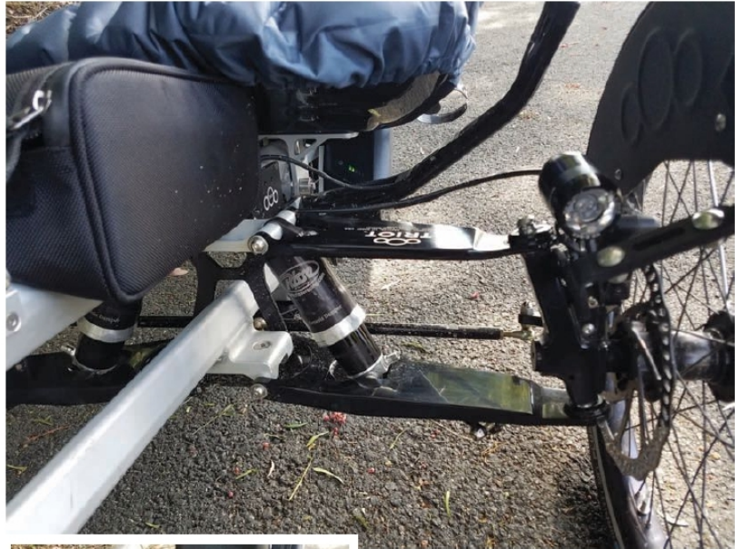
Above: Front suspension showcases more examples of beautiful machine work and design and provides a delightful ride. Left: Seating on the Triot is a unique inflatable bladder design over a padded carbon-fiber shell.
