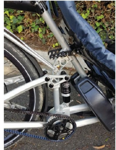
Above and below: Supple rear suspension and dual a dual battery help supply a comfortable ride for long distances.
