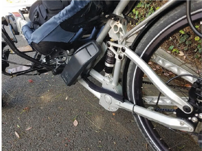
Above and below: Supple rear suspension and dual a dual battery help supply a comfortable ride for long distances.
